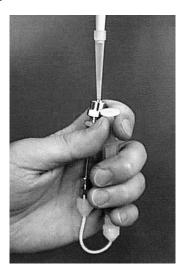
Repeat these steps until a pre-column is totally filled with the gel. The precolumn has to be filled completely in the precolumn and is better to be slightly over filled. Then tighten the two parts by wrench. The filter can easily fell off from the precolumn. Please pay caution to avoid it.
