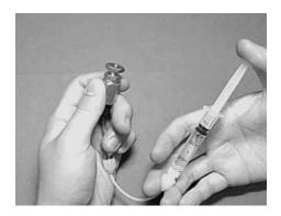
After these steps connect the pre-column to the HPLC system (normally before the column after injectors, before injector in the case of microdialysis samples). First connect tube only to the up stream side and wash inside by pumping mobile phase. After several minutes connect tube to the down stream side too. Except for microdialysis, failure of pack of pre-column makes shapes of peaks strange.
